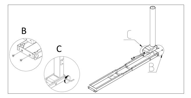
**Step 3**Install the table feet Screws 4 pcs M6x35,install the 4 leveling pads.
